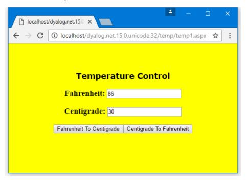
The TemperatureConverterCtll control contains other standard controls as child controls. A control that acts as a container must implement an interface called INamingContainer.
